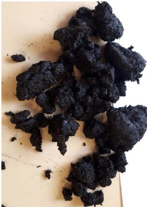
Plate 1: WS105B 1.2-1.7m BGL, peat deposit (image from SOCOTEC 2018)
